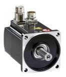
servo motor BMH, Lexium 32, 34.4Nm, 3800rpm, keyed shaft, without brake, IP65, IP67, 128bit encoder, straight
