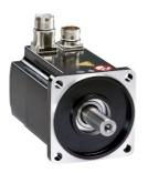
servo motor BMH, Lexium 32, 62.5Nm, 3800rpm, keyed shaft, without brake, IP54, 128bit encoder, straight
