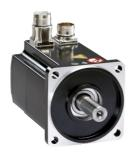
servo motor BMH, Lexium 32, 62.5Nm, 3800rpm, untapped shaft, without brake, IP65, IP67, 16 multiturn encoder, straight
