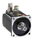
servo motor BMH, Lexium 32, 62.5Nm, 3800rpm, untapped shaft, with brake, IP65, IP67, 16 multiturn encoder
