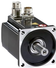
servo motor BMH - 84 Nm - 3800 rpm - untapped shaft - with brake - IP54
