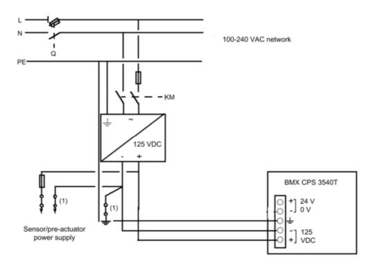
**Q** General isolator **KM** Line contactor or circuit breaker
