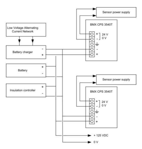
125 VDC floating network for the power supply of sensors, actuators and input/out modules. Connection of Direct Current Power Supply Modules to an Alternating Current Network
