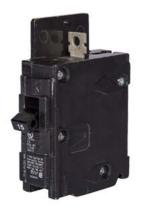
Siemens Low Voltage Molded Case Circuit Breakers General Purpose MCCBs are Circuit Protection Molded Case Circuit Breakers. 1-Pole circuit breaker type BQH. Rated 120V (025A) (AIR 22 kA). Special features: Load side lugs are included.
