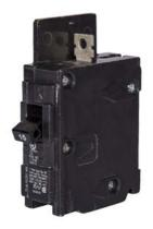
Siemens Low Voltage Molded Case Circuit Breakers General Purpose MCCBs are Circuit Protection Molded Case Circuit Breakers. 1-Pole circuit breaker type BQH. Rated 120V (070A) (AIR 22 kA). Special features: Load side lugs are included.
