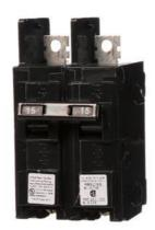
Siemens Low Voltage Molded Case Circuit Breakers General Purpose MCCBs - Type BQ, 2-Pole, 120/240VAC are Circuit Protection Molded Case Circuit Breakers. 2-Pole Common-Trip circuit breaker type BQ. Rated 120/240V (015A) (AIR 10 kA). Special features: Load side lugs are included.
