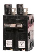
Siemens Low Voltage Molded Case Circuit Breakers General Purpose MCCBs - Type BQ, 2-Pole, 120/240VAC are Circuit Protection Molded Case Circuit Breakers. 2-Pole Common-Trip circuit breaker type BQ. Rated 120/240V (025A) (AIR 10 kA). Special features: Load side lugs are included.
