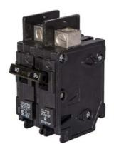
Siemens Low Voltage Molded Case Circuit Breakers General Purpose MCCBs - Type BQ, 2-Pole, 120/240VAC are Circuit Protection Molded Case Circuit Breakers. 2-Pole Common-Trip circuit breaker type BQH. Rated 120/240V (025A) (AIR 22 kA). Special features: Load side lugs are included.
