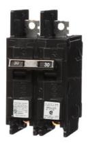
Siemens Low Voltage Molded Case Circuit Breakers General Purpose MCCBs - Type BQ, 2-Pole, 120/240VAC are Circuit Protection Molded Case Circuit Breakers. 2-Pole Common-Trip circuit breaker type BQH. Rated 120/240V (030A) (AIR 22 kA). Special features: Load side lugs are included.
