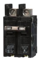
Siemens Low Voltage Molded Case Circuit Breakers General Purpose MCCBs - Type BQ, 2-Pole, 120/240VAC are Circuit Protection Molded Case Circuit Breakers. 2-Pole Common-Trip circuit breaker type BQ. Rated 120/240V (030A) (AIR 10 kA). Special features: line side lugs included. Note: Load side lugs are included.
