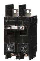
Siemens Low Voltage Molded Case Circuit Breakers General Purpose MCCBs - Type BQ, 2-Pole, 120/240VAC are Circuit Protection Molded Case Circuit Breakers. 2-Pole Common-Trip circuit breaker type BQ. Rated 120/240V (090A) (AIR 10 kA). Special features: Load side lugs are included.
