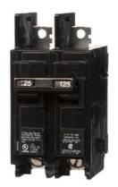
Siemens Low Voltage Molded Case Circuit Breakers General Purpose MCCBs - Type BQ, 2-Pole, 120/240VAC are Circuit Protection Molded Case Circuit Breakers. 2-Pole Common-Trip circuit breaker type BQ. Rated 120/240V (125 A) (AIR 10 kA). Special features: Load side lugs are included.
