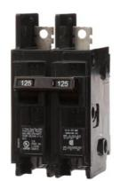
Siemens Low Voltage Molded Case Circuit Breakers General Purpose MCCBs - Type BQ, 2-Pole, 120/240VAC are Circuit Protection Molded Case Circuit Breakers. 2-Pole Common-Trip circuit breaker type BQH. Rated 120/240V (125 A) (AIR 22 kA). Special features: Load side lugs are included.
