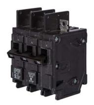
Siemens Low Voltage Molded Case Circuit Breakers General Purpose MCCBs are Circuit Protection Molded Case Circuit Breakers. 3-Pole Common-Trip circuit breaker type BQH. Rated 240V (070A) (AIR 22 kA). Special features: Load side lugs are included.
