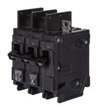
Siemens Low Voltage Molded Case Circuit Breakers General Purpose MCCBs are Circuit Protection Molded Case Circuit Breakers. 3-Pole Common-Trip circuit breaker type BQH. Rated 240V (090A) (AIR 22 kA). Special features: Load side lugs are included.
