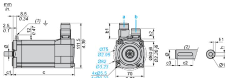
a: Power supply for servo motor brake
