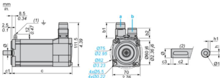
a: Power supply for servo motor brake
