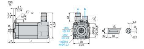
a: Power supply for servo motor brake
