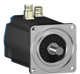
AC servo motor BSH, Lexium 05, 3.4N.m, 2500rpm, untapped shaft, with brake, IP50
