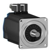
servo motor BSH, Lexium 05, 5.5N.m, 4000rpm, 100mm, keyed shaft, Sincos single turn, without brake, IP50
