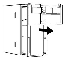
3. Slide in the Communications Board in slit and press it all the way to the back.
