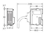
8/6-point Basic I/O Units, Interrupt Input Unit, and Highspeed Input Unit
