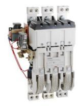
Mechanically held lighting contactor, Contactor amp rating 400A, 0 N.C. / 3 N.O. poles, 110VAC 50HZ/120VAC 60HZ coil, Non-combination type, Enclosure NEMA type (open), No enclosure
