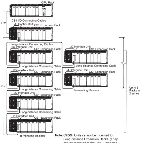
Long-distance Expansion Racks. (They can be mounted to the CS1 Expansion Rack with the I/O Control Unit mounted.)
