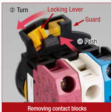
Removing contact blocks
