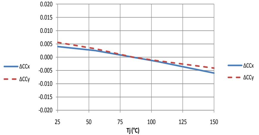
The following graphs represent typical chromaticity vs current and temperature for the XLamp CXA2011 at **5000K** CCT.
