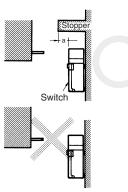
Refer to *Dimensions* for the mounting dimension of the Operation Key and mount the Operation Key correctly. The Operation Key will soon become damaged or worn out if it is not mounted correctly.
