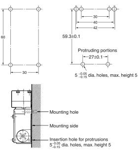
The D4BS can be mounted more securely by adding two protruding portions, each of which is 5 mm maximum in height and 5  $^{-0.05}$ /\_\_0.16 mm in diameter as shown below.
