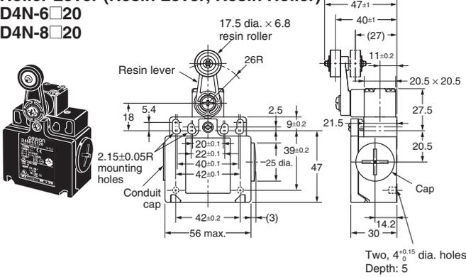
**Roller Lever (Metal Lever, Resin Roller)**
