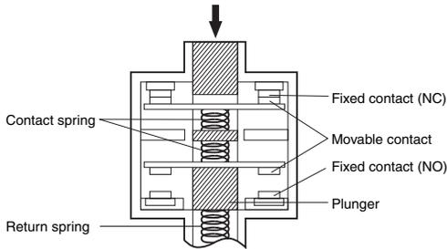
Conforms to EN60947-5-1 Direct Opening Operation ⊖
