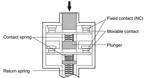
Conforms to EN60947-5-1 Direct Opening Operation ⊖
