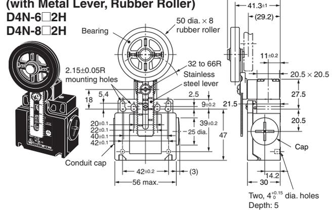
Note: Unless otherwise specified, a tolerance of ±0.4 mm applies to all dimensions.
