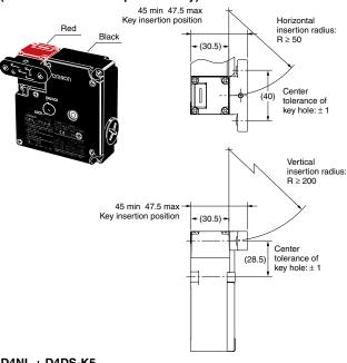
D4NL + D4DS-K5 (with Front-inserted Operation Key)
