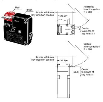
D4NL + D4DS-K1 (with Top-inserted Operation Key)
