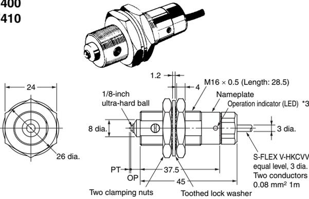
M16 Type (Contact Output/Solid-state Output)
