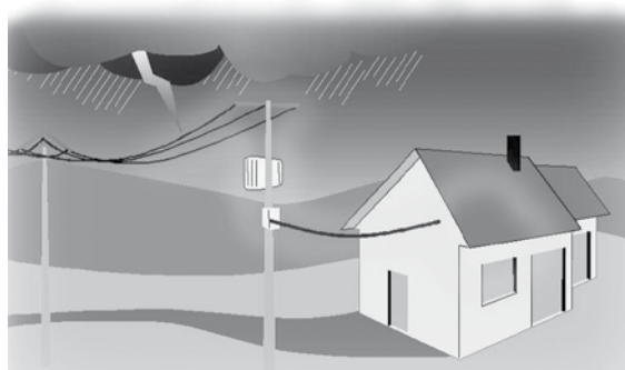
Direct lightning strike on an overhead line
