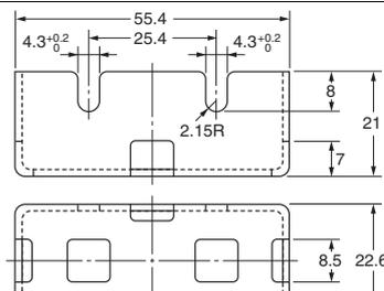
Note: The Cover has six holes for easy lead wire connections.
