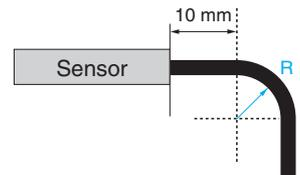
\* For a robot (bending-resistant) cable, multiply the bending radius in the above table by 1.7.
