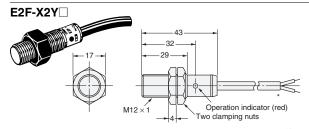
\* 6-dia. vinyl-insulated round cable with 2 conductors (Conductor) cross section: 0.5 mm<sup>2</sup>, Insulator diameter: 1.9 mm), Standard length: 2 m
