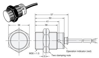
6-dia, vinvl-insulated round cable with 2 conductors (Conductor cross section: 0.5 mm², Insulator diameter: 1.9 mm), Standard length: 2 m
