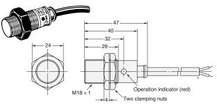
\* 6-dia. vinyl-insulated round cable with 2 conductors (Conductor cross section: 0.5 mm², Insulator diameter: 1.9 mm), Standard length: 2 m
