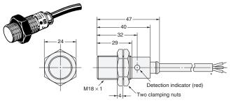
\* 6-dia. vinyl-insulated round cable with 3 conductors (Conductor cross section: 0.5 mm², Insulator diameter: 1.9 mm), Standard length: 2 m
