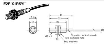
\* 3.5-dia. vinyl-insulated round cable with 2 conductors (Conductor cross section: 0.14 mm², Insulator diameter: 1 mm), Standard length: 2 m The cable can be extended up to 200 m (separate metal conduit).
