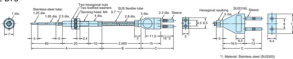
Note 1. The maximum allowable temperatures for sections A, B, and C are 400°C, 300°C, and 110°C, respectively. The section inserted into the Amplifier Unit (indicated by \*2), however, must stay within the Amplifier Unit's operating temperature range.
