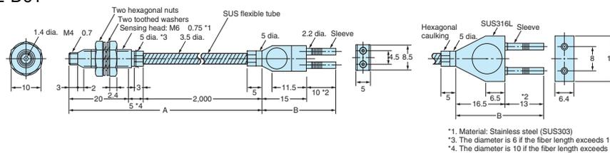
Note 1. The maximum allowable temperatures for sections A and B are 350°C and 110°C, respectively. The section inserted into the Amplifier Unit (indicated by \*2), however, must stay within the Amplifier Unit's operating temperature range.
