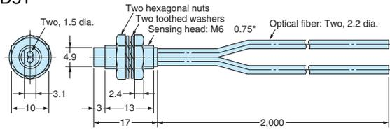
Note: The maximum allowable temperature is 150°C. The maximum allowable temperature for continuous operation is 130°C.
