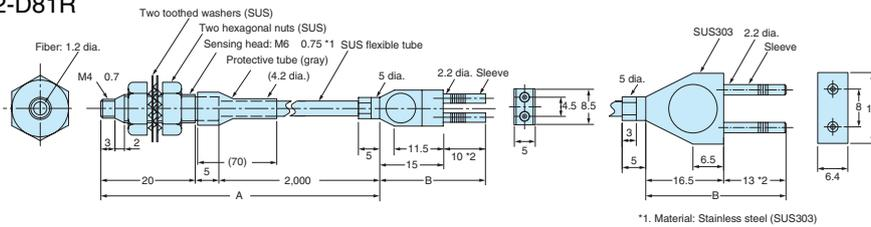
Note 1. The maximum allowable temperatures for sections A and B are 200°C and 110°C, respectively. The section inserted into the Amplifier Unit (indicated by \*2), however, must stay within the Amplifier Unit's operating temperature range.
