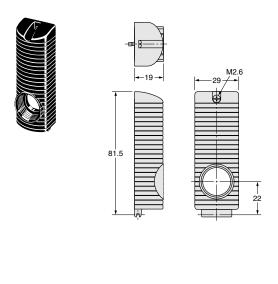
Note: 1 . The cover is provided with a rubber bushing and cap to prevent the cable from being pulled out in vertical direction.
