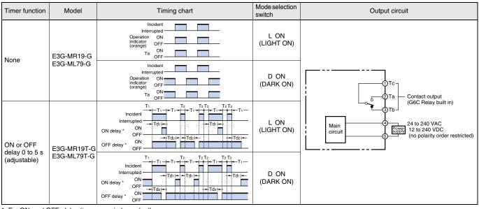
\* For ON and OFF, delay timers vary independently. Note: Td1, Td2: Delay time (0 to 5 s), T1: Any period longer than delay time, T2: Any period shorter than delay time
