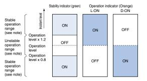
Note: If the operation level is set to the stable operation range, the E3G will operate with the highest reliability and without being influenced by temperature change, voltage fluctuation, dust, or setting change. Maximum distance setting (in normal mode)
