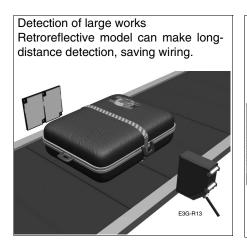
Detection of large corrugated cardboard Just by installing the sensor on one side, only the boxes to be detected shall be sensed.
