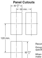
Recommended panel thickness is 1 to 8 mm. Group mounting is not possible. (Maintain the specified mounting space between Controllers.)
