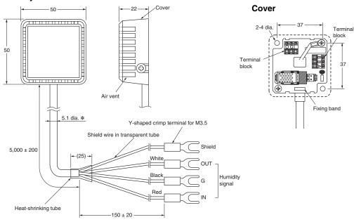
The above figure is for the ES2-HB-N. The ES2-THB-N has temperature output wires (yellow/green/brown).
