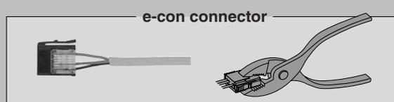
**No need to strip the wire** Only pliers are required for clamping.
