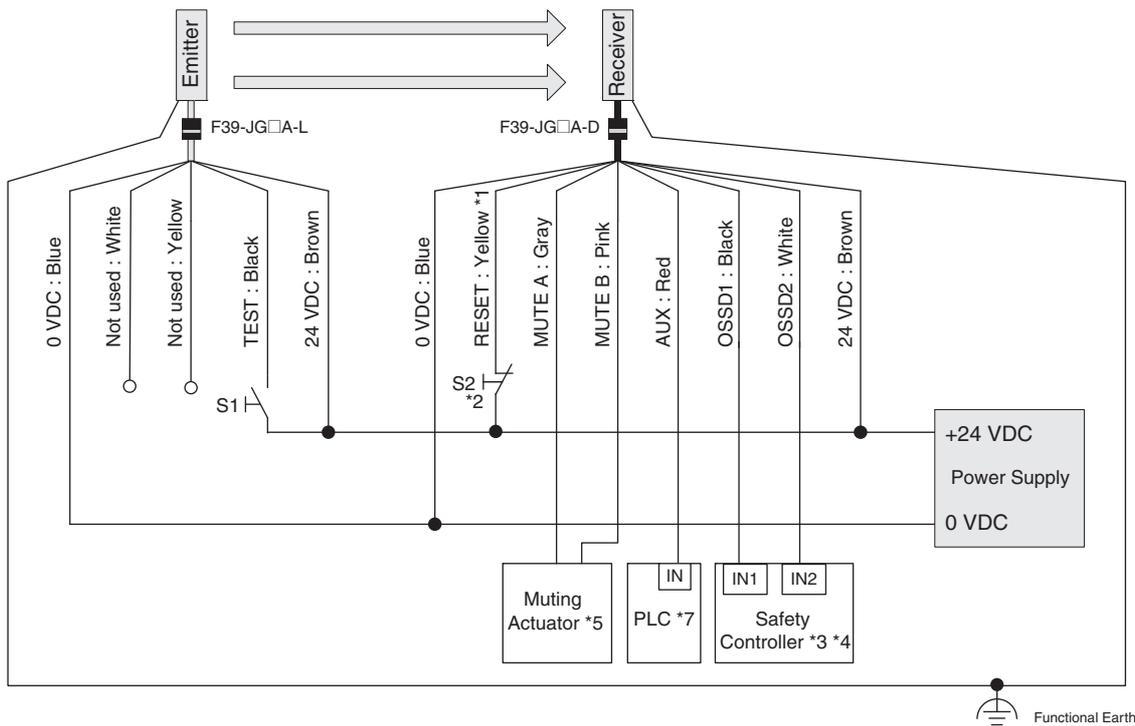
S1: Test Switch (Connect the line to 0 V if this switch is not required)
