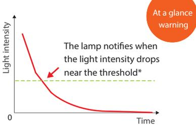
\* The incident light level at which the light curtain turns OFF
