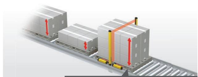
\* Partial muting: A function that allows specified beams (e.g., beams blocked by a workpiece) to be disabled, keeping others active, even during muting.
