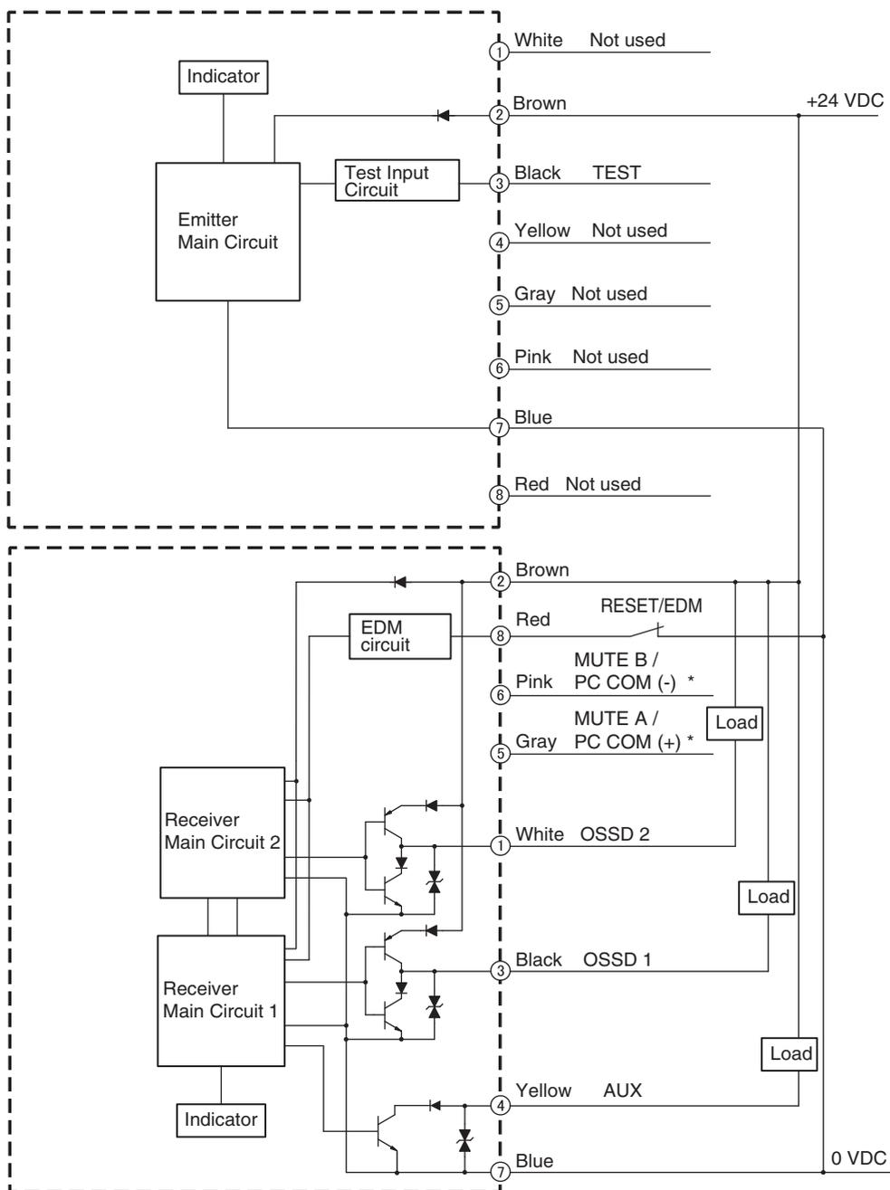
\* This line is used for communication with a PC using the F39-GIF-1 Interface Unit.
