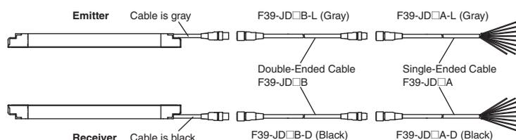
**Cascading Cable (2 cables per set, for emitter and receiver)**
