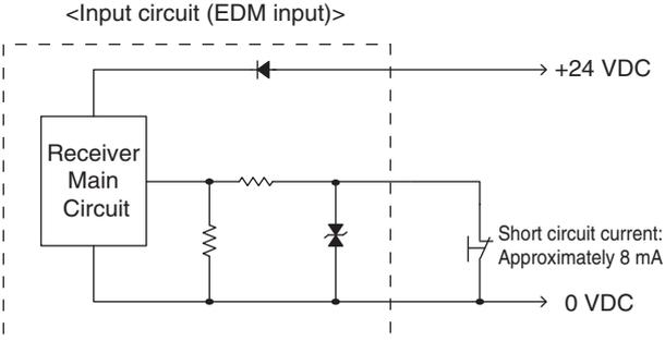
\*Short circuit current: 5mA (Reset input), 3mA (Muting inputs A/B)
