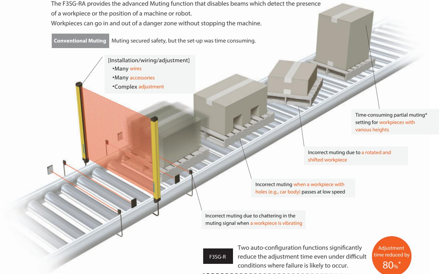
**F3SG-R** Two auto-configuration functions significantly reduce the adjustment time even under difficult conditions where failure is likely to occur.
