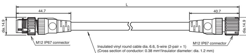
Double-Ended Cable for Receiver: Cable for extension (F39-JG□B-D, sold separately)
