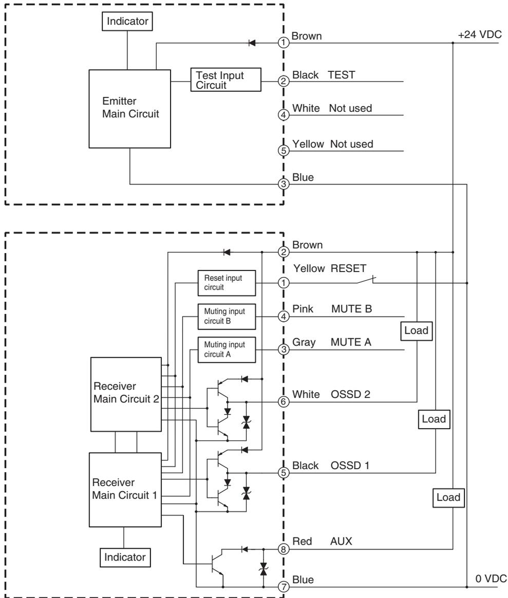
**Input Circuit Diagram by Function**
