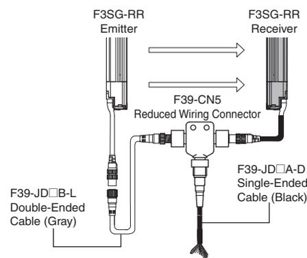
**Cable for Reduce Wiring\* (2 cables per set, one for emitter and one for receiver)**
