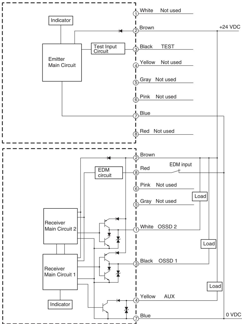
**Input Circuit Diagram by Function**
