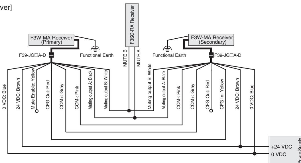
**Note:** The wiring examples in later pages do not indicate functional earth. To use functional earth, wire an earth cable according to the example above. Refer to *Smart Muting Actuator F3W-MA Series User's Manual* for more information.
