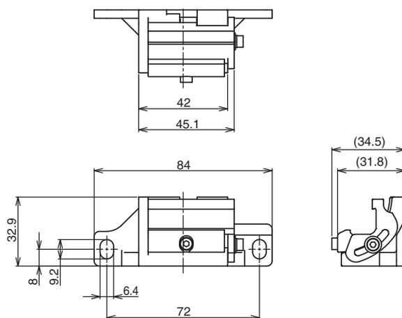
Material: Zinc alloy, Fluorochemical lubricant oil
