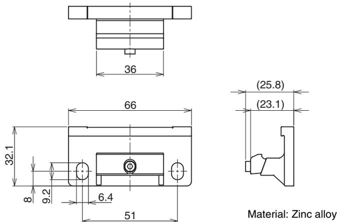
Mounted with F3W-MA Bracket (F39-LGMA□) and Standard Adjustable Bracket (F39-LGA) on F3SG-RA
