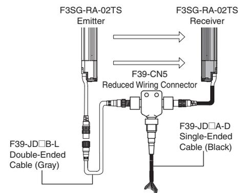
**Cable for Reduce Wiring\* (2 cables per set, one for emitter and one for receiver)**
