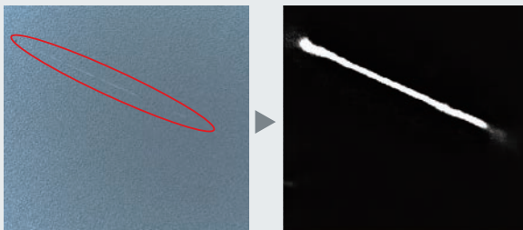
Scratch on sandblasted metal
