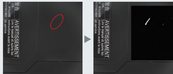
Scratch on resin products
