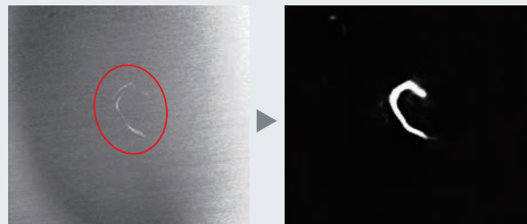
White scratch on shaded hairline finish
