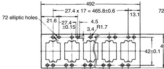
Note: PYP-18 and PYP-36 can be cut to a desired length for mounting less than 18 or 36 Sockets, respectively.
