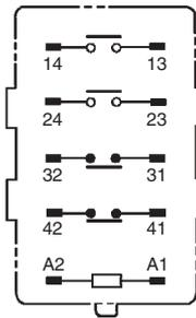
**Note:** Terminals 43 and 44 of the G7J-4A-P(T) and contacts 41 and 42 of the G7J-3A1B-P(B) are bifurcated contacts.
