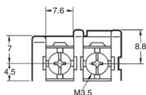
Allow suitable slack on leads when wiring, and do not subject the terminals to excessive force.
