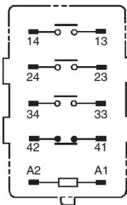
The coil has no polarity.
