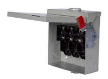
Siemens Low Voltage Circuit Protection General Duty Safety Switches. Type: ENCLOSED, SAFETY SWITCH Std: UL V. Rating: 240VAC/120VAC A. Rating: 60A No. Of Poles: 2P F. Rating: 60Hz Action: SINGLE THROW Material: 304SS Enclosure: TYPE 3R. 2-3 point mounting holes. O. Cycles: 10000 O. Temperature: (-20F-120F) AMBIENT TEMPERATURE Environmental Conditions: OUTDOOR
