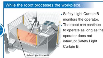
**Note:** If the operator is able to completely enter the zone inside Safety Light Curtain B, a presence detection device, such as a Safety Mat, is necessary as an additional safety measure.
