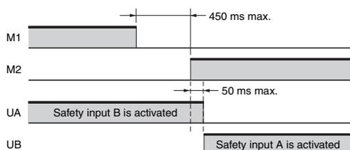
(When M1 turns OFF after M2 turns ON)
