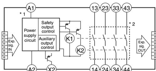
\*1. Internal power supply circuit is not isolated.
