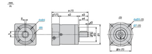
(1) Dimensions a, a1, c, Ø6 and Ø7 depend on the planetary gearbox/servo motor combination
