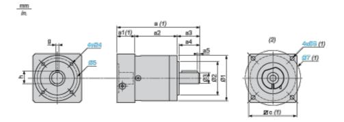
(1) Dimensions a, a1, c, Ø6 and Ø7 depend on the planetary gearbox/servo motor combination
